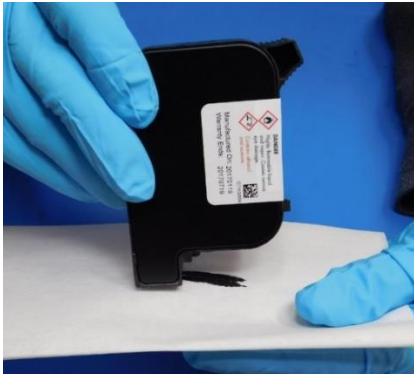
Figure 6 - Finger supported wiping method
