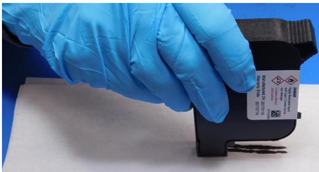
Figure 4 – “Wicking wipe” technique for removing hardened deposits of ink and debris (initial wipe)
