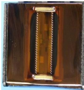
Figure 2 - Image of an orifice plate after maintenance wiping with a dry, lint-free wipe
