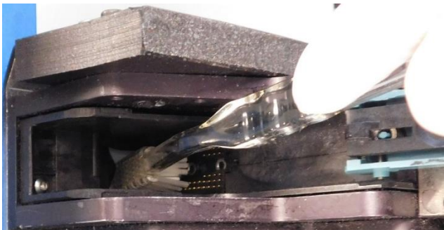
Figure 11 – Using a toothbrush to clean the cartridge stall
