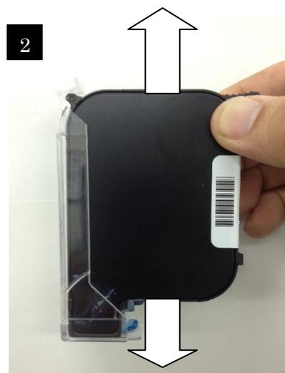
3. After shaking the cartridge, please remove the clip and wipe excess ink with a lint-free dry cloth from the print head facing down.
