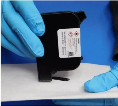
Figure 6 - Finger supported wiping method
